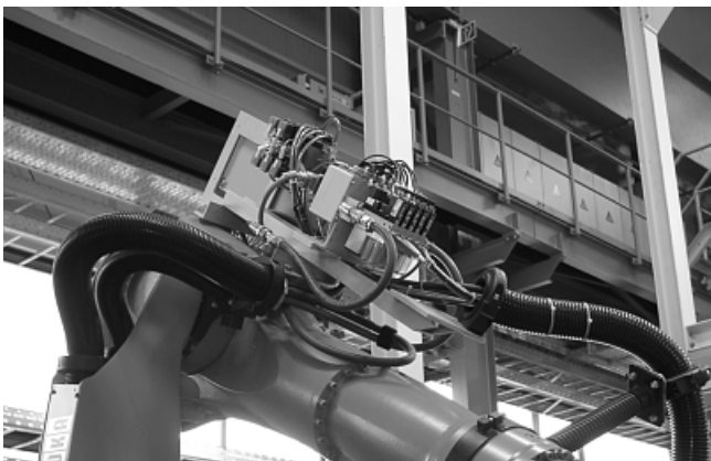
Vacuum generator on a robot arm, consisting of five compact ejectors SMP
