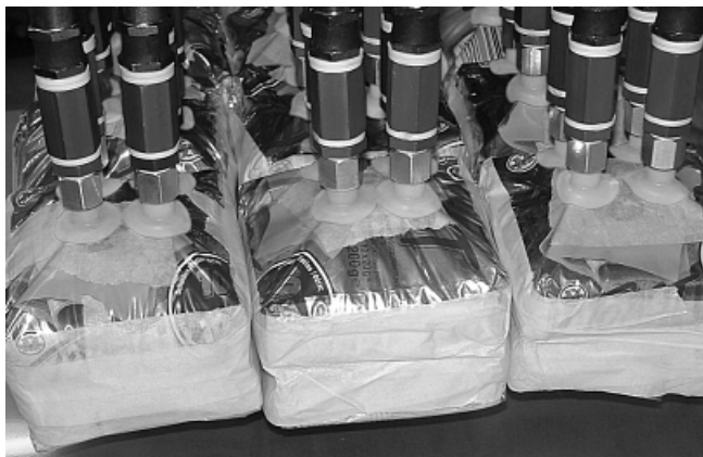
Foil and paper suction pads SGPN SI being used for handling blister packs
