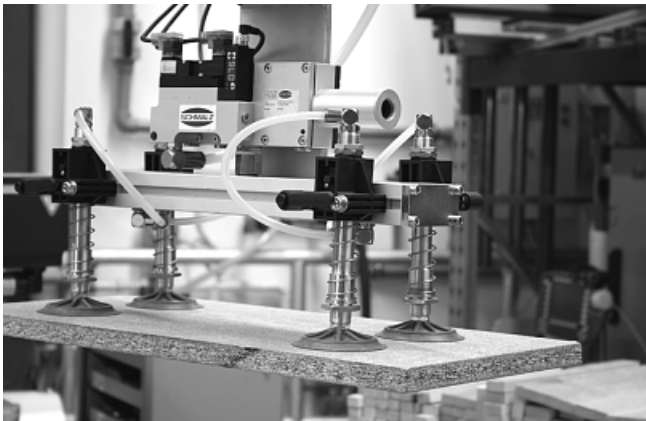
Vacuum cross-beam with vacuum generation by means of a regulated multi-stage ejector SEM-C for handling of chipboard sheets
