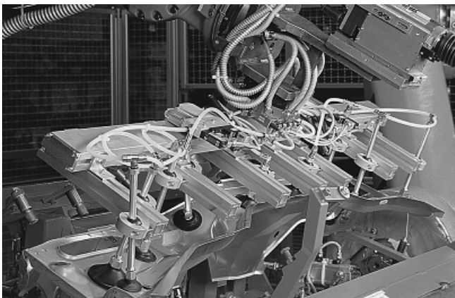
Vacuum generator on a vacuum spider for handling metal sheets
