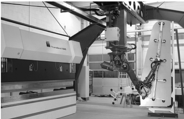
Vacuum spider with flat suction pads SAF for automatic loading of a folding press with sheets of metal
