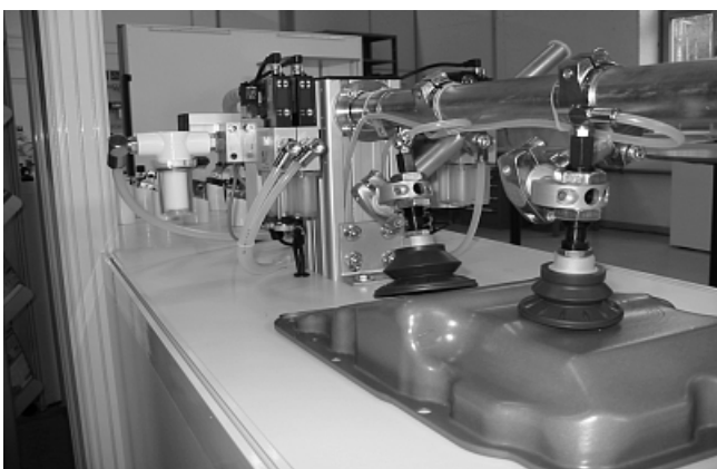
Mounting example HTR-FST A3 on a vacuum spider
