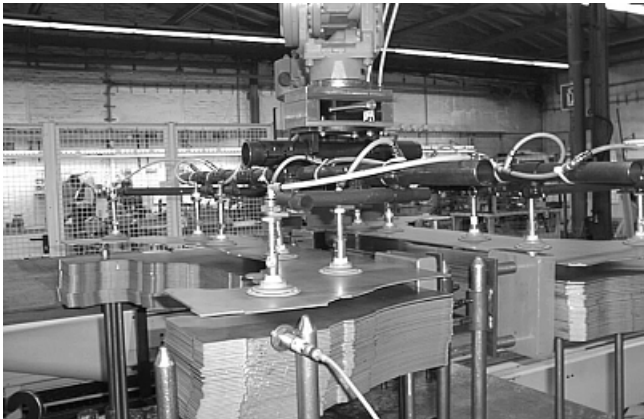
Spring plungers FSTE-HD on a vacuum spider for handling of sheet metal in the automobile industry
