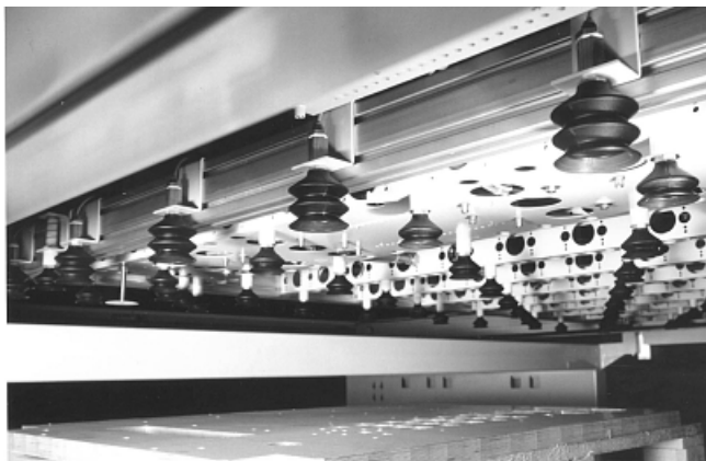
Wear-resistant bellows suction pad FSGA VU1 for handling of sheet metal
