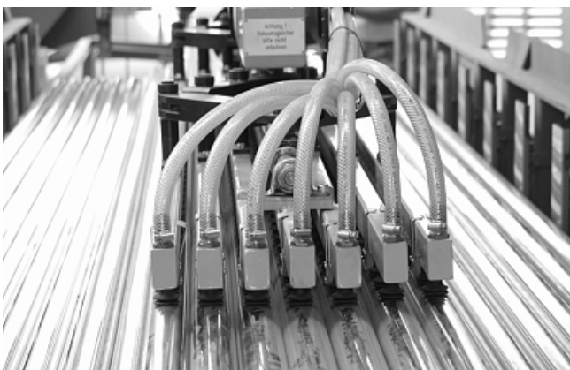
Handling of pipes with adaptable bellows suction pads FSG
