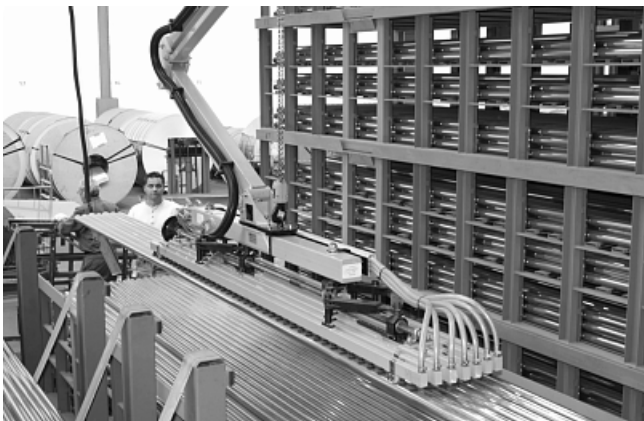
Handling of pipes with adaptable bellows suction pads FSG and FSGB
