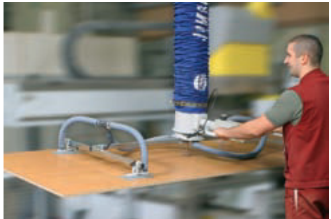
JumboErgo, maximum load 85 kg, with multiple vacuum gripper, for loading and unloading CNC woodworking machines
