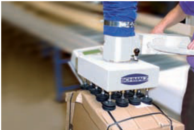
JumboErgo, maximum load 45 kg, with multiple vacuum gripper Compact, for handling non-rigid cardboard boxes
