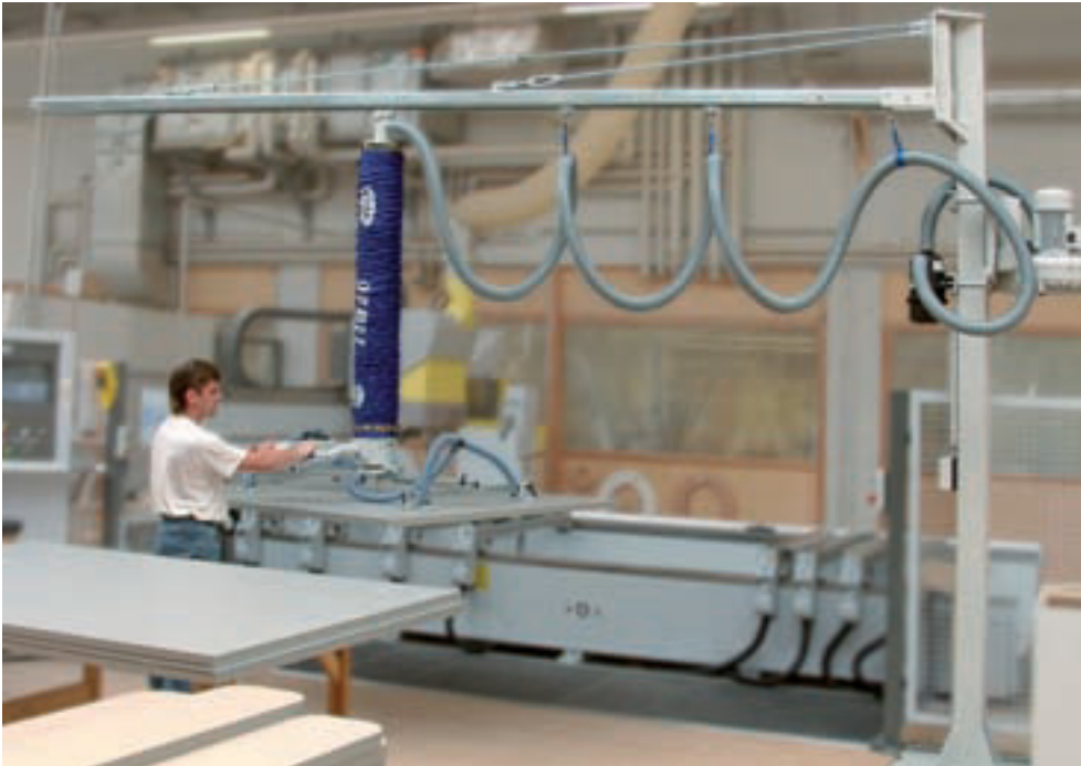
Jumbo Ergo, maximum load 85 kg, with double suction pad, for loading and unloading a CNC woodworking centre
