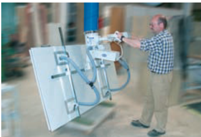
Jumbo Ergo, maximum load 90 kg, with pneumatic swivelling unit and quadruple suction pads, for handling sheets of wood
