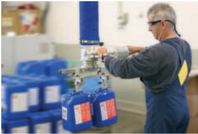
JumboErgo, maximum load 45 kg, for unstacking canisters on a roller conveyor
