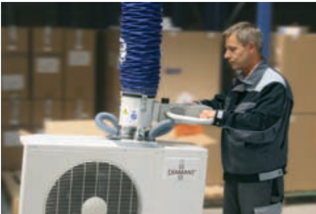
JumboErgo, maximum load 85 kg, with double suction pad, for handling air-conditioning units
