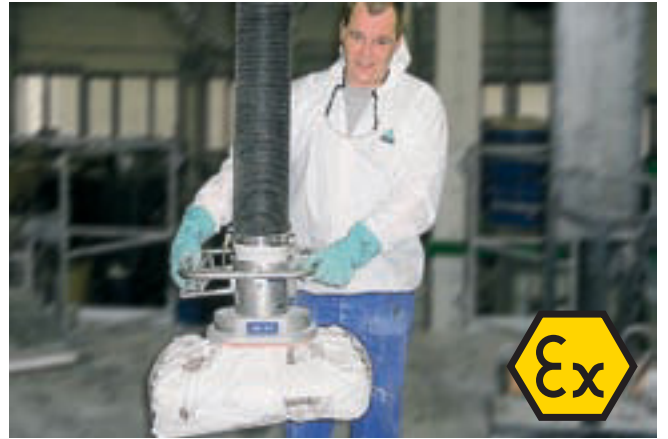
JumboSprint, maximum load 65 kg, with sack gripper, for handling sacks in explosion-hazard areas to ATEX
