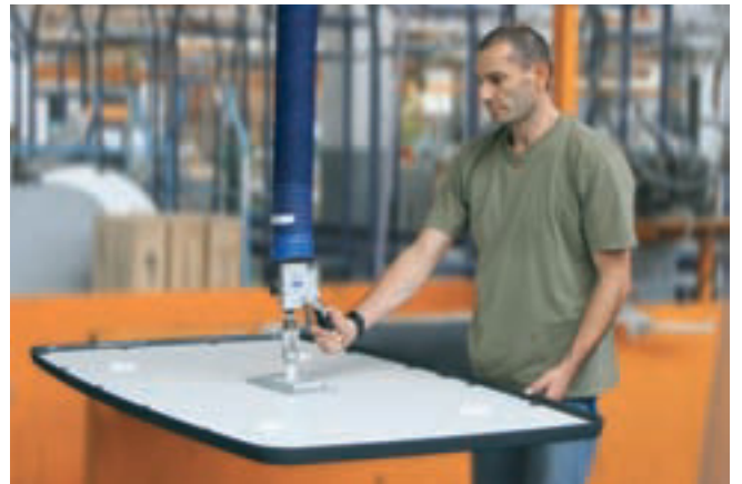
JumboHandy, maximum load 30 kg, with single suction pad for commissioning camping tables
