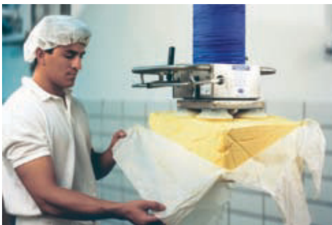
JumboSprint, maximum load 65 kg, stainless steel, for handling foodstuffs in the food industry
