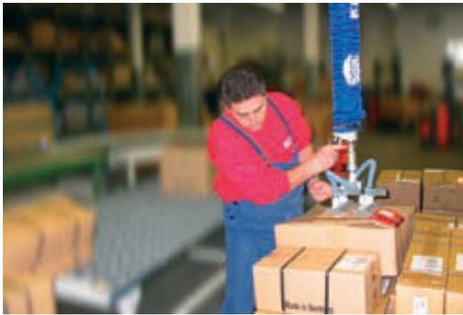
JumboHandy, maximum load 30 kg, with double suction pad, for handling cardboard boxes
