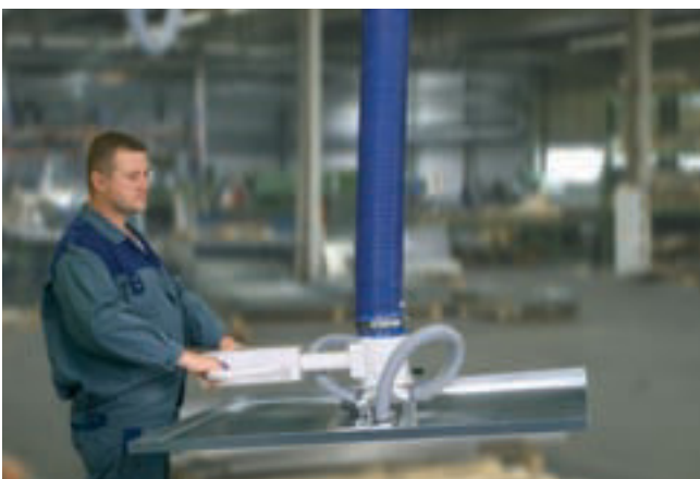
JumboErgo, maximum load 45 kg, with double suction pad, for loading gluing machines
