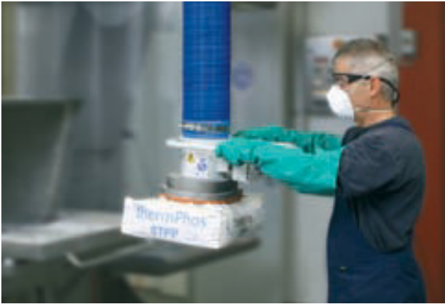
Jumbo Sprint, maximum load 45 kg, with sack gripper, for handling plastic and paper sacks
