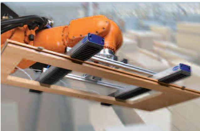
Large-area vacuum gripping system FXC for handling of doors
