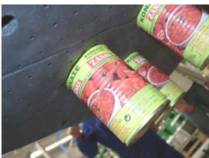
Vacuum gripper system SPZ for layer handling of cans
