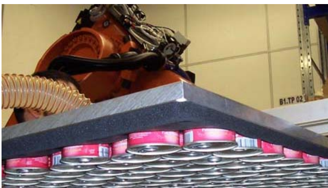
Vacuum gripper system SPZ for layer handling of cans
