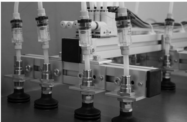
Inline filter VFI on a vacuum spider to protect the vacuum generators
