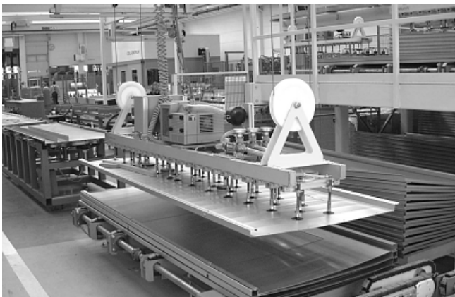
Solenoid valves EMV for control of vacuum in segments of a vacuum cross-beam
