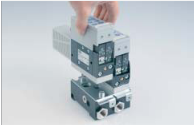
Quick changing of SXP pumps on a dual block
