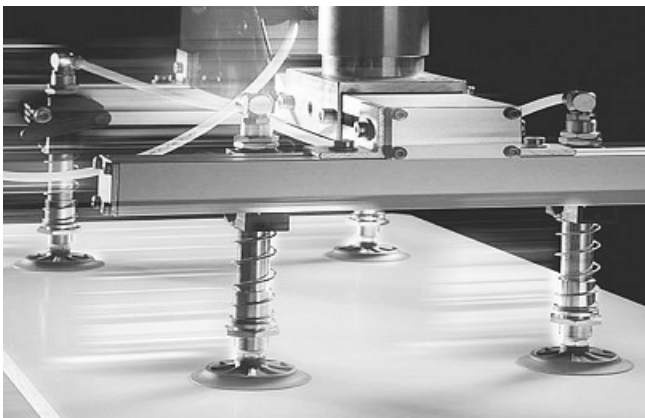
Vacuum gripper equipped with spring plungers FSTF for handling wood panels
