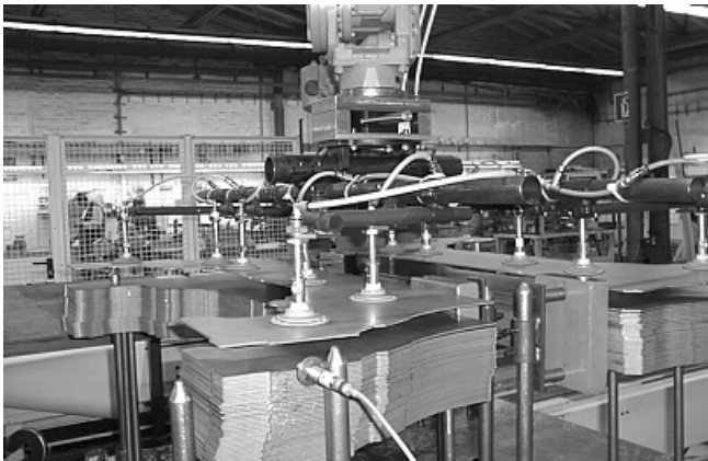
Spring plungers FSTE on a vacuum spider for handling of sheet metal in the automobile industry
