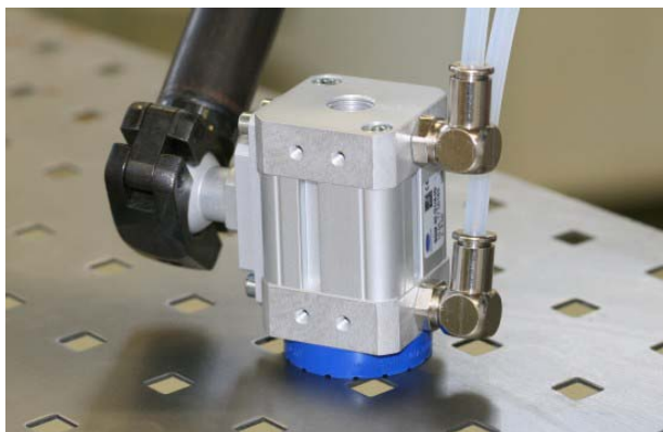
Gripper spider with magnetic grippers SGM being used to handle perforated sheets of metal
