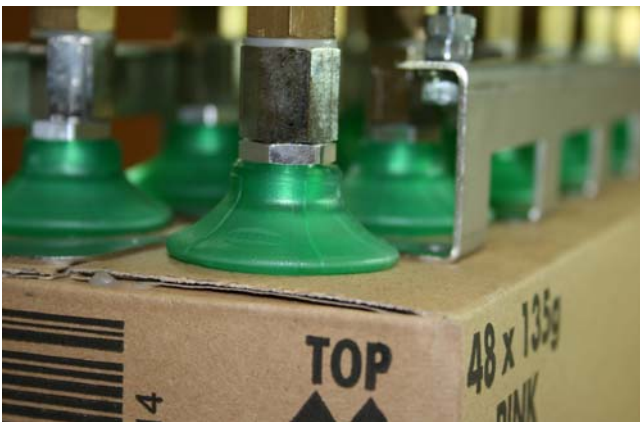
Bellows suction pads SPB1 for handling of cardboard boxes
