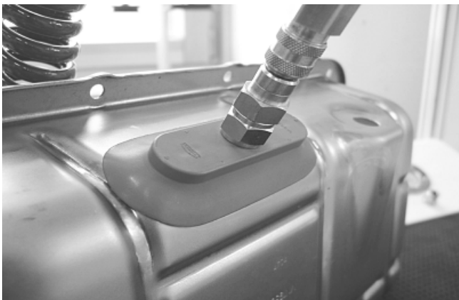
Bell suction pad SAOG for lifting very curved sheet-metal parts
