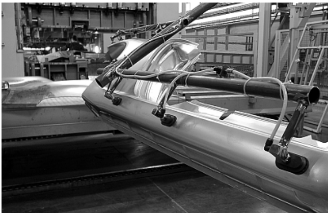
Vacuum spider with bellows suction pads SAOB for handling bodywork parts in the automobile industry
