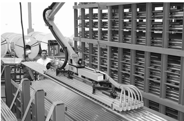
Handling of pipes with adaptable bellows suction pads FSG and FSGB
