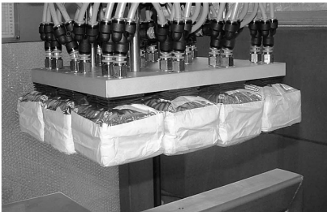
Bellows suction pad FSGB-R for handling of easily damaged packing materials
