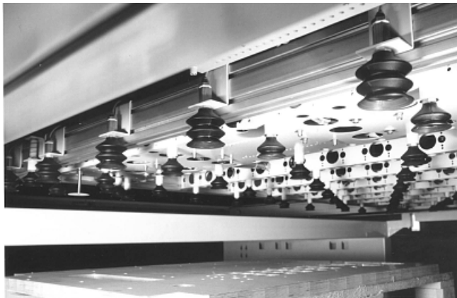
Wear-resistant bellows suction pad FSG VU1 for handling of sheet metal
